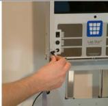
Carefully punch a hole for the camera; remove wrap by unlocking security clip. Push the camera gently through the bracket and foam; connect the camera to the monitor
