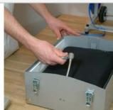
Put the sleeve on top of cover plate; bend camera mount on top of sleeve; place cover on box
