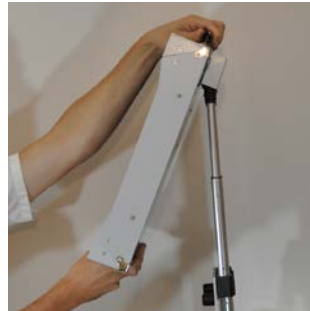
Take box of the trolley, position both. Take and slide the monitor fully over trolley handle
